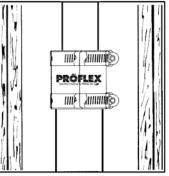
Support pipe and pressure test\* for leaks before concealing joint.
