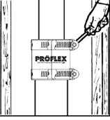
Tighten clamps to 60 inch-lbs. or torque.
