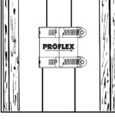
Slide Proflex coupling over the plain spigot ends of the two pipe.
