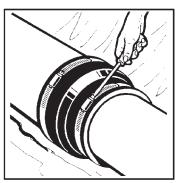
Insert the plain spigot end of the PVC pipe into the other end of the flexible coupling.
