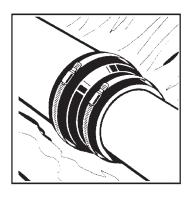
Slide flexible coupling over the end of the corrugated drain pipe, making sure to get the corrugation past the rib on the inside of the coupling.
