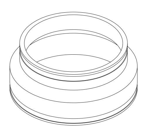
Equipped with 300SS Clamps Installation Torque 60in-lb
