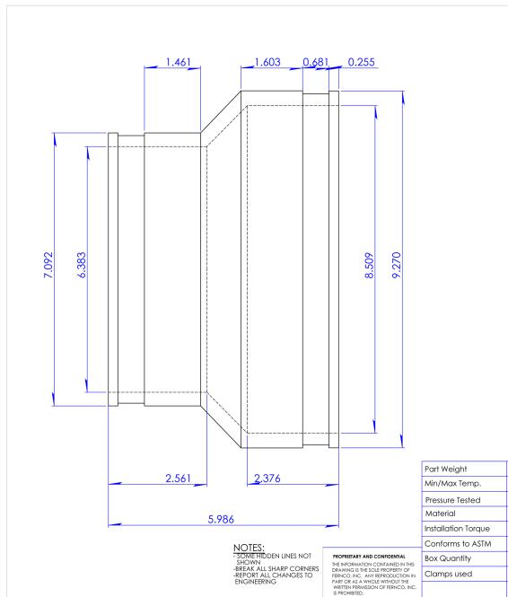
\* Part is flexible and will stretch or tighten down approx. 5% of ID size.
