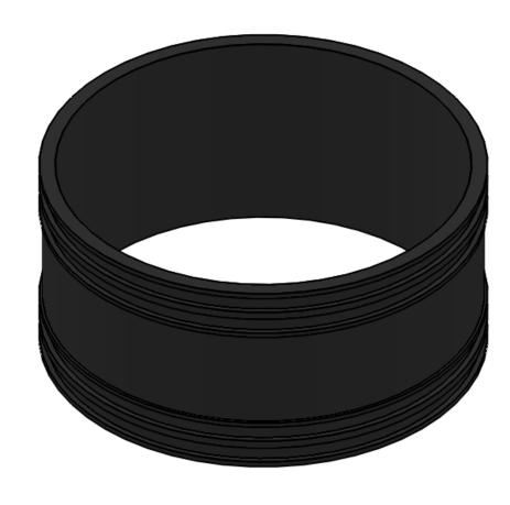
"RC" Shield: .012 x 5.00 x 62" 300SS w/2 Standard Clamps Installation Torque 60 in-lb
